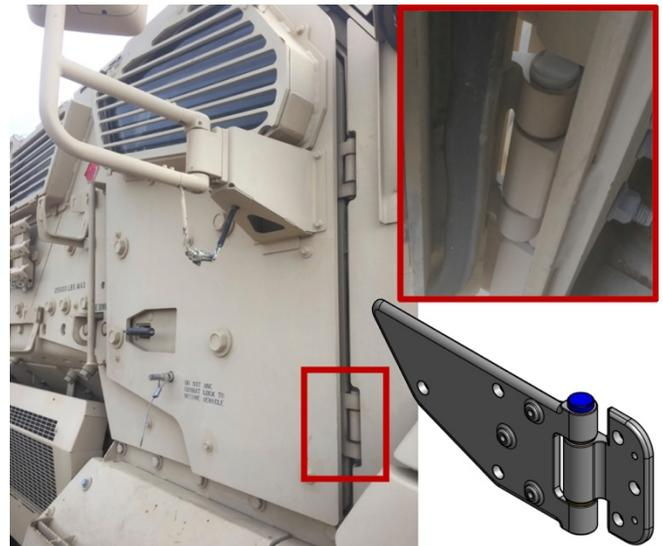
**Figure 1.** MAXXPRO MRAP showing location and CAD model of door hinge assembly.
